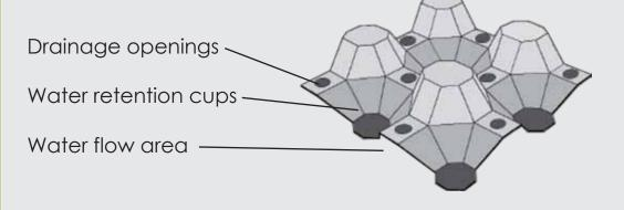
GRS 1.5 is a great drainage and water retention layer for any green roof application. The rigid plastic is strong enough to handle heavy loads yet there is enough open space to allow water to flow freely to drains. The resevoir cups hold water to help with the storm water retention capacity of the green roof system.
